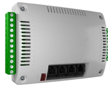
Figure 14. VAV controller for demand-controlled ventilation
