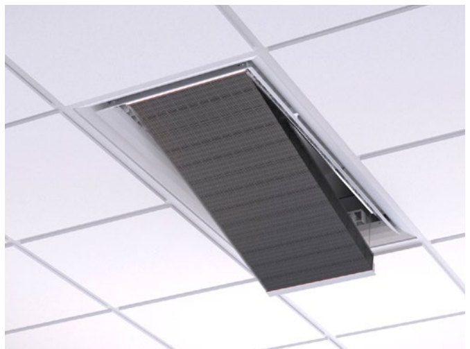
Figure 13. Removing the face plate and folding out the coil for accurate cleaning in the event of high hygiene requirements. Note! requires the product to be ordered with the accessory, fold-out coil, and that flexible connection hoses are used on the water side.
