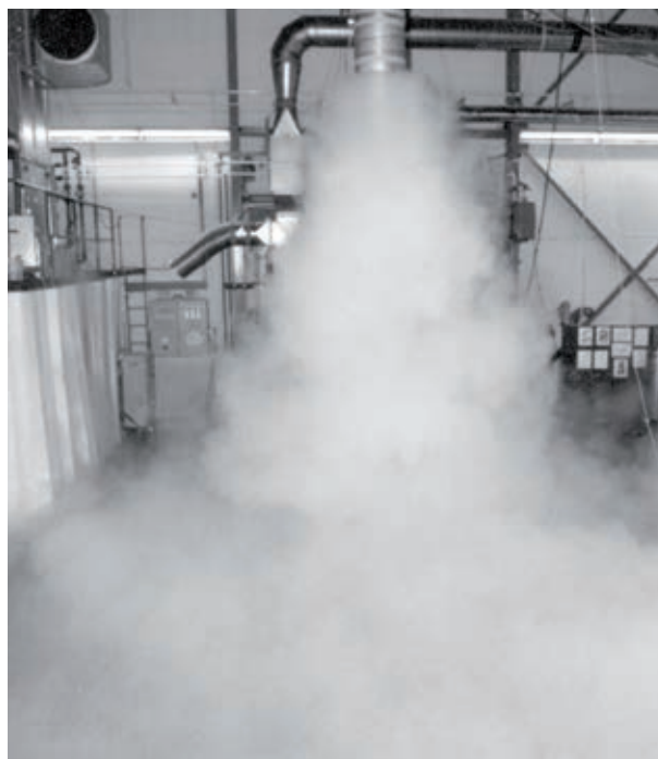
Fig. 5: Air jet dispersion made visible by smoke tracer top: cooling mode bottom: heating mode
