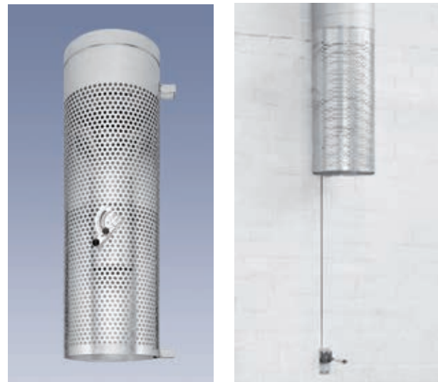
Fig. 2: Circular displacement outlet with adjustable damper left: adjustment with control lever right: adjustment with Bowden cable
