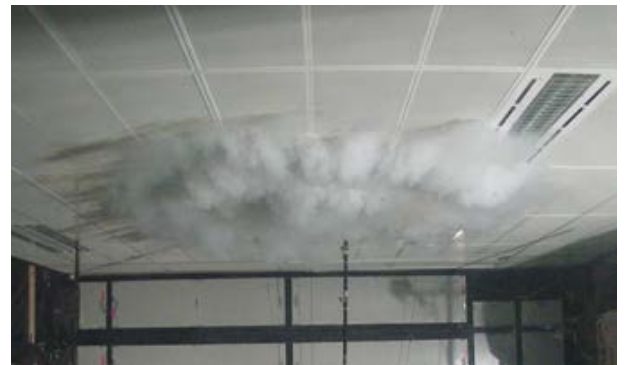
Figure 1: Air flow pattern made visible by smoke tracer
