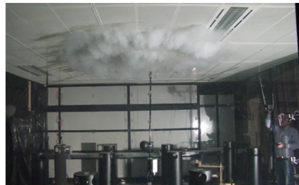
Fig. 2: Flow pattern of the Opticlean made visible by smoke
