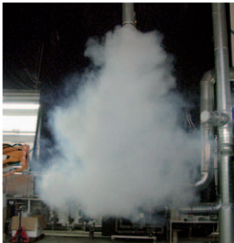
Fig. 3: Jet spread when cooling and heating, made visible by smoke tracer
