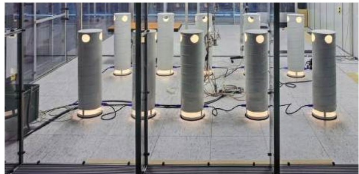
Heat and cooling output test cabin
